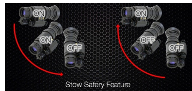
Stow Safety Feature, SSF : built-in electronic solution to help an operator stay covert during night-time operations: turns off the IIT when it is rotated up or down in the vertical plane.
