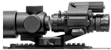
Zero Lens Kit ZL (transforms PBS14 into a clip-on night vision sight to be mounted in front of daytime optical sight. Kit comes with weapon mount and an additional 3X Afocal objective lens).
